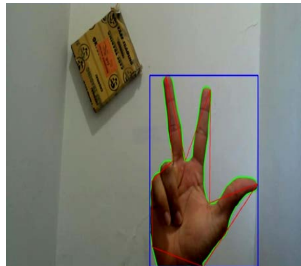
Figure3: After applying the Convex Hull algorithm for ASL based Gesture digit 3.
