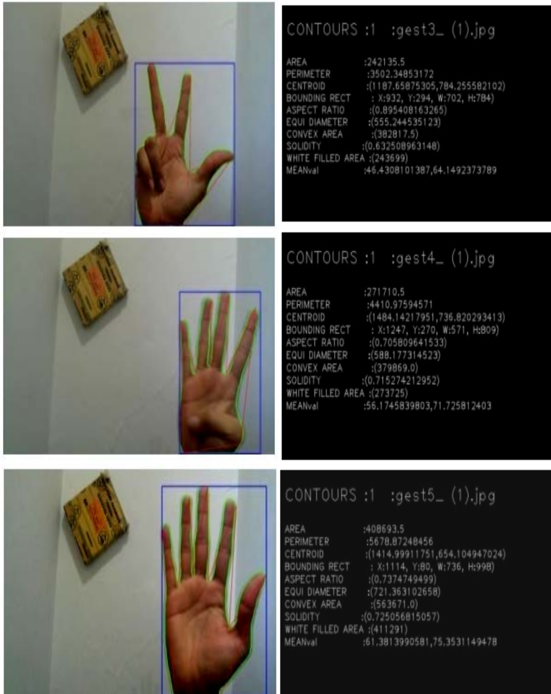
Figure 5: Segmentation of hand with Bounding rectangle and polygon.
