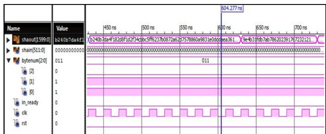
Figure 15: HDL simulation result of keccak hash function with pipelining
