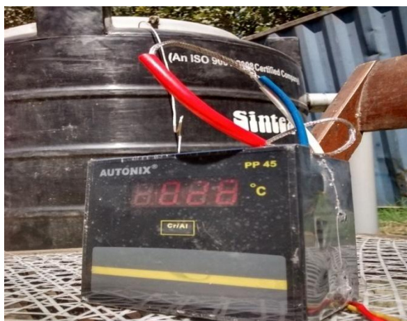
Figure 1: Thermocouple for temperature measurement
