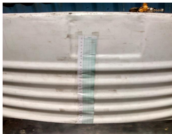
Figure 2: Graph scale to measure rising height of floating drum
