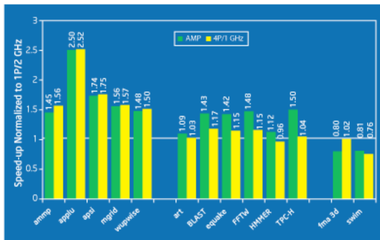
Figure 5: Comparison of speedup with SMP and AMP using highly parallel programs (left), moderately.
