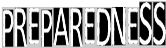
Fig 6.1.5: Detection of connected components of a string
