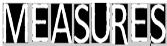
Figure 6.1.7: Detection of connected components of a string
