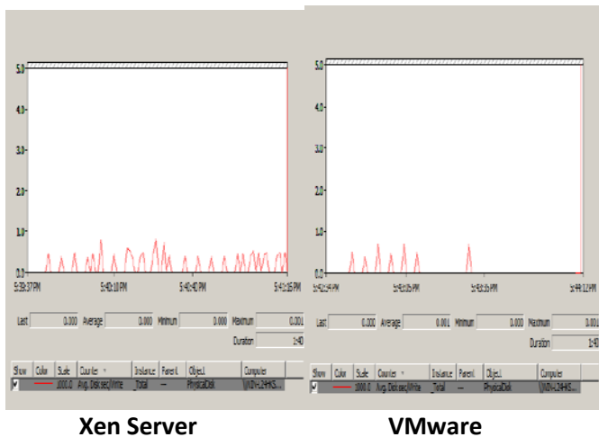
Figure 7: Disk write rate frequency comparison of VMware ESXi and XenServer
