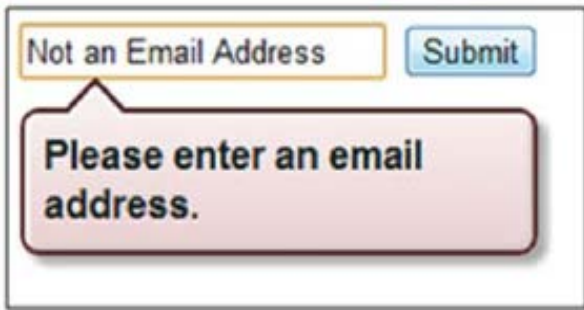
Figure 9: Page that uses the code for the simple form validation with HTML5. [1]
